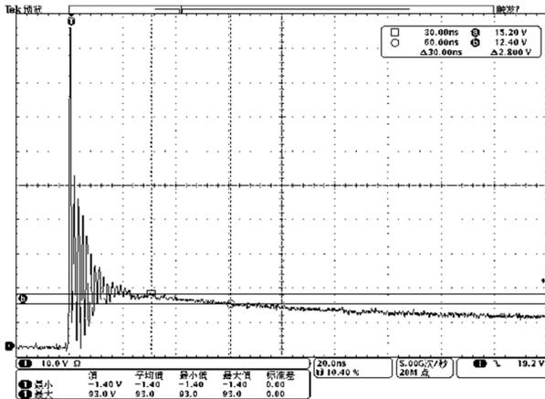
Fig 7. Clamping Voltage at IEC61000-4-2 +8kV Pulse Waveform
