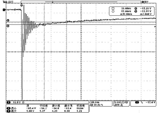
Fig 8. Clamping Voltage at IEC61000-4-2 -8kV Pulse Waveform
