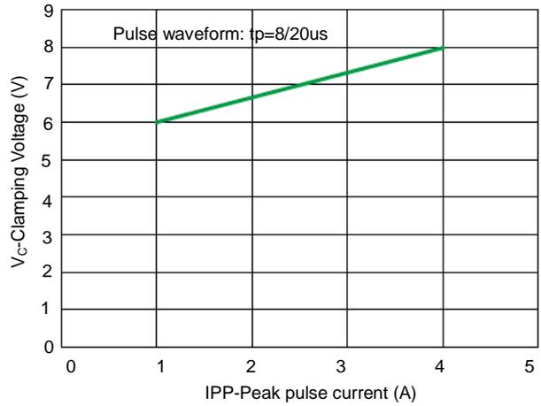
Fig 2. Clamping voltage vs. Peak pulse current
