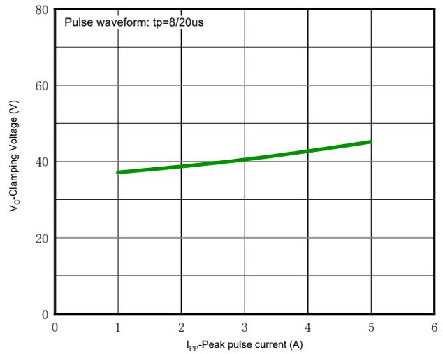
Fig 4. Clamping voltage vs. Peak pulse current
