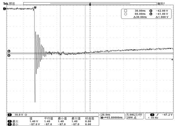
Fig 8.ESD Clamp[ing voltage] (IEC61000-4-2 -8KV contact)
