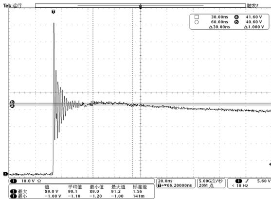
Fig 7.ESD Clamp[ing voltage] (IEC61000-4-2 +8KV contact)
