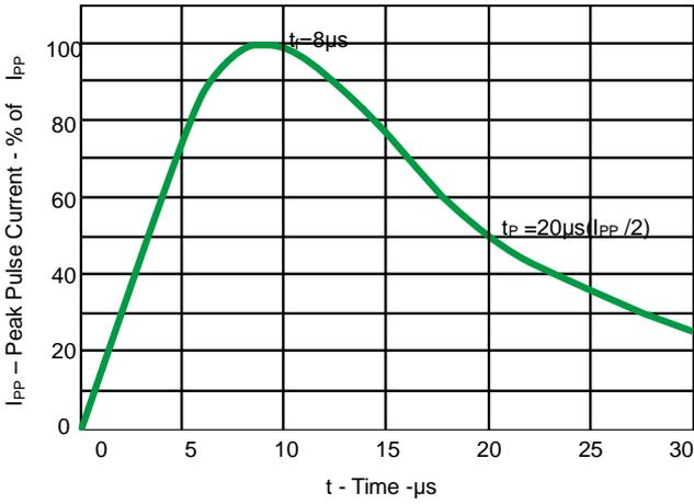
Fig 1. Pulse Waveform
