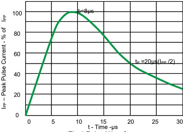
Fig 1. Pulse Waveform
