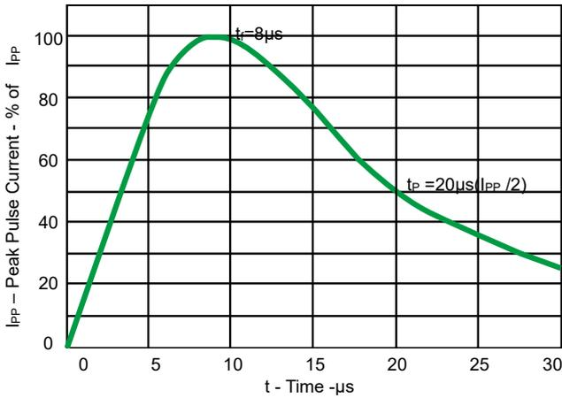
Fig 1. Pulse Waveform
