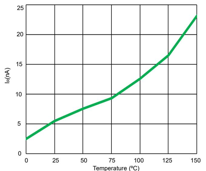
Fig 6. Typical Leakage Current vs. Temperature
