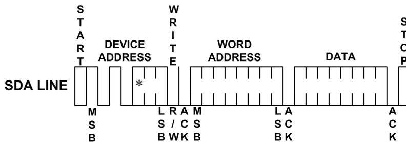
Figure 5: Byte Write
