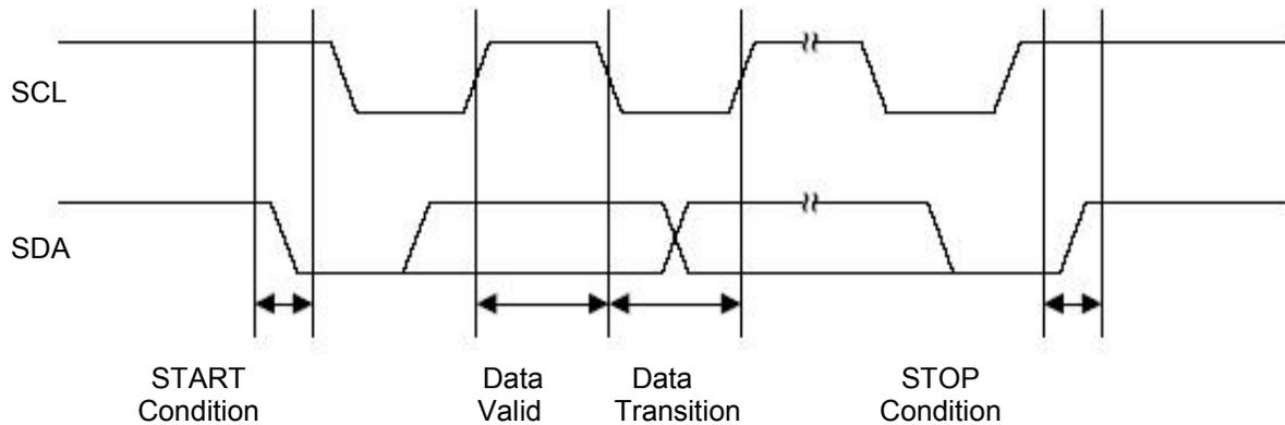
Figure 3: Timing diagram for START and STOP conditions
