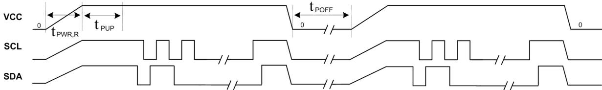
If an event occurs in the system where the VCC level supplied to the device drops below the maximum  $V_{POR}$  level specified, it is recommended that a full power cycle sequence be performed by first driving the VCC pin to GND, waiting at least the minimum  $t_{POFF}$  time and then performing a new power-up sequence in compliance with the requirements defined in this section.
